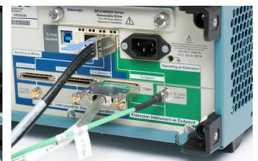
UltraSync connection on instrument with Extension role
