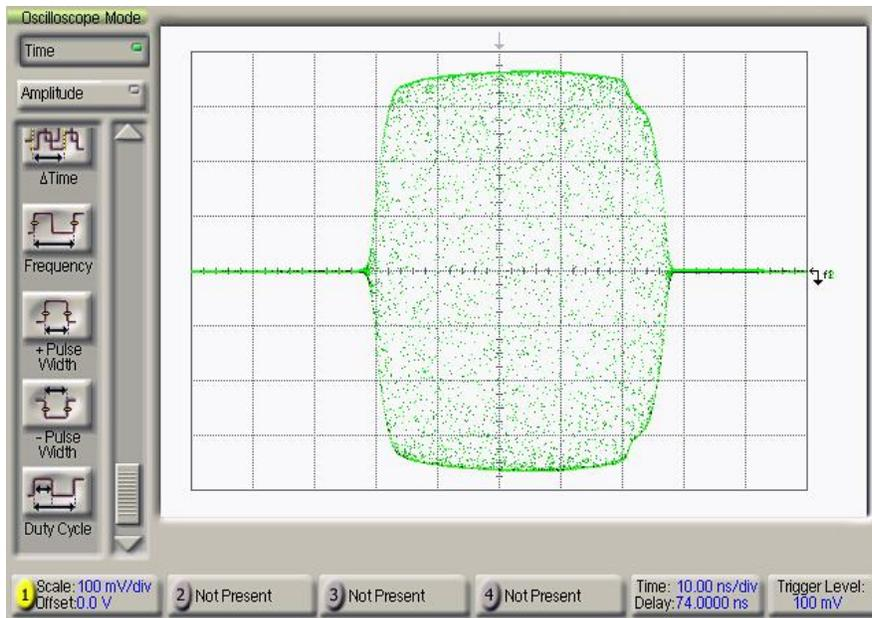
**Figure 3.** Measured pulse shape; Frequency = 9 GHz, power = 5 dBm, amplitude = 5 dBm, ALC off, pulse width = 50 ns, pulse period = 200 ns. The oscilloscope is protected by a 10 dB pad and the timescale is set to 10 ns/div.
