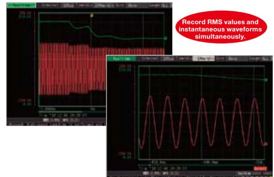
Record RMS values and instantaneous waveforms simultaneously.
